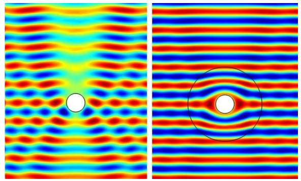
Invisibility cloaking illustrating how cloaking works using electromagnetic cloaking. On the left, electromagnetic waves, which could be light, scatter upon hitting the cylinder in the middle. On the right, the cylinder is cloaked; the waves do not scatter, and to a beholder standing on the field, it would appear invisible. Credit: Creative Commons,
