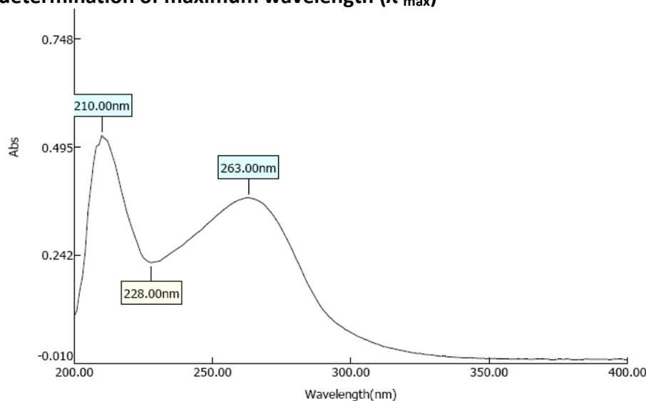
Fig. 2: UV spectrum of Lurasidone.
