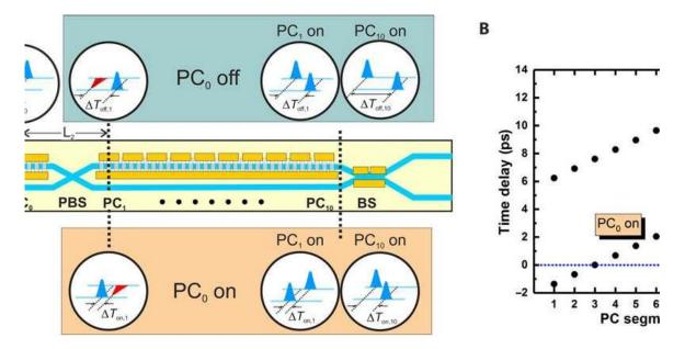
Illustration of the principle of the adjustable BED line. (A) The diagram shows the chip design together with some insets illustrating the temporal relation of the horizontally (red) and vertically (blue) polarized photon wave packets at ...more
