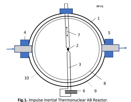
*Notations*: 1 - strong spherical body (shell) of reactor (diameter about  $0.3 \div 3$  m); 2 – the special fuel capsule (it is
