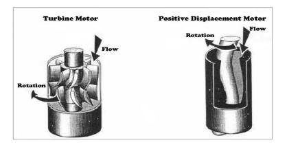
Figure1-the directional drilling motors with circulation
