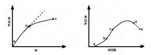
Figure2-the relation between the permeability rate of rock and the rotary speed of the equipments and the weight on the bit
