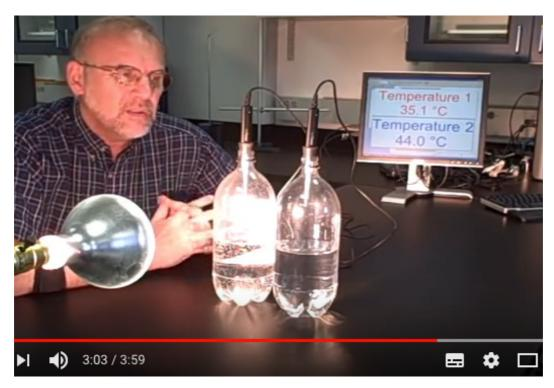
**Figure 39. Greenhouse Gas Bottle Demonstration [82].** Bottles with CO2 and air are radiated and temperature measured – CO2 in blue. Is this not an experiment to measure the heat capacities of the respective gases?
