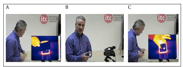
Figure 30. Demonstrating with the thermal imaging camera: (A) 'opaque' thermoelectric glass in front of the heat source; (B) visibly opaque germanium in hand; (C) 'transparent' non-thermoelectric germanium placed in front of heat source [55].
