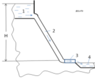
Fig. 10. Typical Hydroelectric station with ABJEG. Notations: 1 - upper source; 2 - water canal; 3 – ABJEG; 4 – lower runoff.
