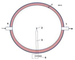
**Fig. 2**. AB thermonuclear electric impulse reactor. *Notations*: 1 - strong spherical body (shell) of reactor (diameter about 0.3 - 3 m); 2 - the fuel cartridge (it is described in Fig.1); 3 - holder of fuel cartridge; 4 - enter of compressed air (gas); 5 - exit of a hot compressed air (gas) after thermonuclear heating; 6 - electric conductor.
