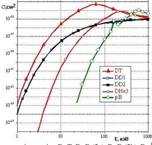
**Fig.4.** Thermonuclear cross section reation D+T, D+D (2a), D+D (2b), D+<sup>3</sup>He, and p+B vs kinetis energy E [keV] of the light particles.
