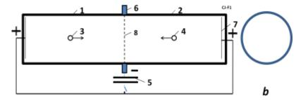
**Fig.1.** Principal schema of the fuel cartrige. *Notation:* a – side view; b – forward view. 1- left fuel camera, 2 - right fuel camera, 3 – thermonuclear fuel in left camera, 4 – themonuclear fuel in right camera (one may be different from left camera), 5 – power electric condenser (50÷150 kJ, voltage 100÷1000 kV), 6 – negative electric contact, 7 –two positive electric contacts, 8 – thin elastic electric conductivity partition.
