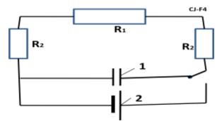
**Fig.5**. Electric schema of connection the condenser to the fuel pellet. *Notation*:  $R_1$  is the resistance of fuel pellet,  $R_2$  is resistance of the connection wires from condenser to the fuel pellet, 1 is condenser, 2 is high voltage electric generator (battery).
