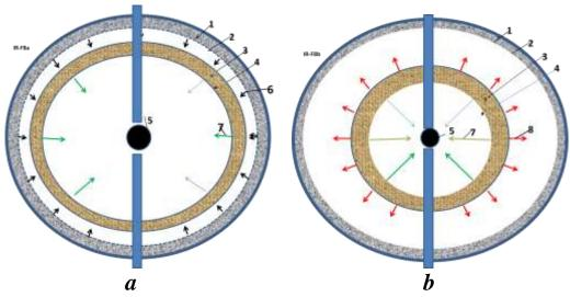
**Fig. 3**. Cumulative canridge of thermonuclear fuel. Work of Cumulative thermonuclear catridge (Version 1). *Notations:* a – initial layer explosive, b – rocket part of explosive. 1 - 5 are same with Fig.3; 6 is pressure of initial layer of explosion, 7 is moving of explosive (force from jetted gas rocket thrust), 8 is flow of reactive explosive gas.
