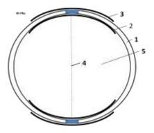
**Fig.5**. Compressed gas pellet for Cumulative and Impulse Thermonuclear reactors. *Notations*: 1- isolator cover; 2, 3 – iternel and externel ejectric contacts; 4 – initial hot ioniser; 5 – compressed gas thermonucler fuel.
