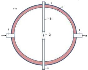
**Fig. 1**. AB thermonuclear cumulative reactor (Version 1). *Notations*: 1- strong spherical body of reactor, diameter about 0.5 - 5 m; 2 – catridge (holder) of fuel pellet, diameter  $1 \div 2$  cm (or pellet inVersion 2, diameter  $2 \div 3$  mm); 3 – holder (electric conductor) of fuel pellet; 4 – enter of compressed air (gas); 5 – exit of a hot compressed air (gas) after thermonuclear heating; 6 – electric voltage.
