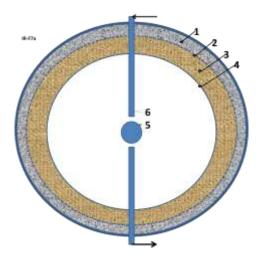
**Fig.2**. Catridge of Cumulative AB-thermonuclear Reactor (Version 1). *Notations*: 1 – strong sphere, 2 – net fusee (electric net), 3 – explosive, 4 - layer (piston) of heavy material, 5 – nuclear fuel (pellet), 6 - electric conductor.
