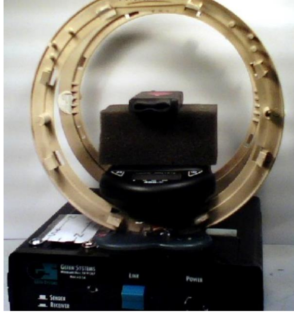
Fig.2. Experiment with VCMS (at the centre) in a uniform (3 mT) field of Helmholtz coils. The VCMS is located on electronic balance, separated by a neutral spacer. The left switch atop of the pedestal changes direction of the external 3 mT field. The red arrow atop of the pedestal changes direction of the external 3 mT field. The red arrow on VCMS shows a direction of its own field.
