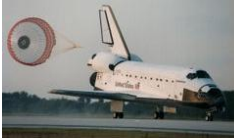
Figure 4-3. Endeavour deploys drag chute after touch-down.
