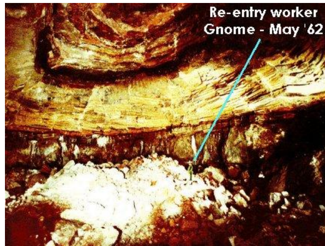
Fig. 1. Project GNOME Rubble Chimney. Look your attention to man into the nuclear underground cavity.
