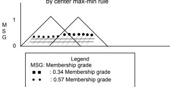
Here, the Centre Max-Min rule is used to find a precise temperature set point by grade of membership(throttle)value.
