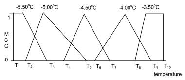
FIGURE 3.5.1: Membership grade of temperature set points
