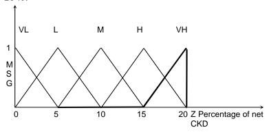
FIGURE 2.3.7: Aggregated output and defuzzification for the percentage of CKD
