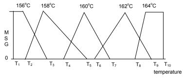
FIGURE 3.4.1: Membership grade of temperature set points
