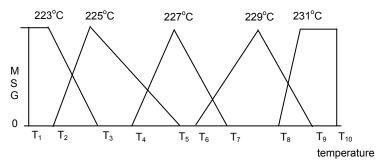
FIGURE 3.3.1: Membership function of temperature set point
