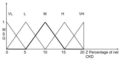
FIGURE 2.3.6: Aggregated output and defuzzification for the percentage of net CKD
