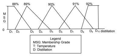
FIGURE 3.3.2: Membership function of percentage of distillation
