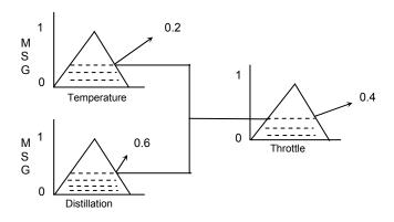
Graph 3.5.4: The two outputs are then defuzzified by center max-min rule
