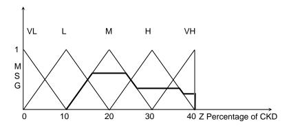
FIGURE 2.2.4: Aggregated output and defuzzificztion for the percentage of CKD
