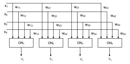
Figure 2.4.2: The feed forward neural network
