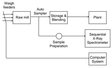
FIGURE 2.4.1 Block schematic of raw mill processing steps
