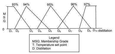
FIGURE 3.4.2: Membership function of percentage of distillation
