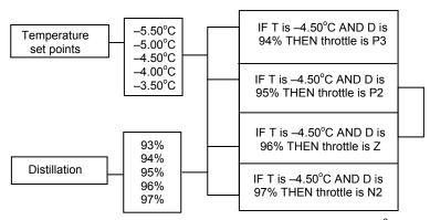
FIGURE 3.5.6: Fuzzy rules for the temperature set point -4.50°C
