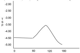
X axis– time in minute and Y axis set point of temperature for naphtha. Set point was –4.50°C
