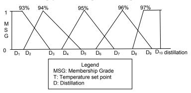
FIGURE 3.5.2: Membership grades of percentage of distillation
