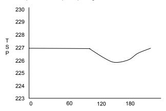
X axis– time in minute and Y axis set point of temperature for Kerosene. Set point was 227°C
