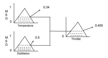
Graph 3.4.2: The two outputs are then defuzzified by center max-min rule
