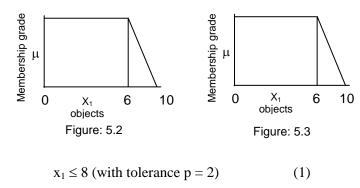
The membership function  $\mu$  are taken along the y-axis i.e.  $\mu(x_1)$  lies in [0, 1] this can be interpreted as the confidence with which this constraint is satisfied (0 for low and 1 for high). The fuzzy inequality constraints can be redefined in terms of their  $\alpha$ -cuts.
