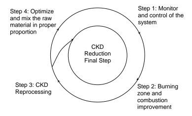
FIGURE 1: CKD Reduction using fuzzy control
