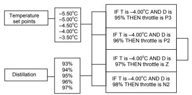
FIGURE 3.5.7: Fuzzy rules for the temperature set point -4.00°C
