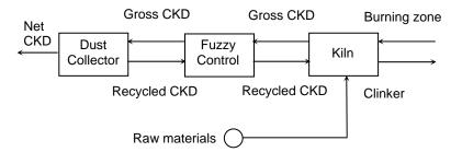
FIGURE 2: Fuzzy control in kiln system
