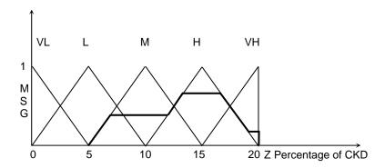
FIGURE 2.3.4: Terms of the output and defuzzification for the percentage of net CKD
