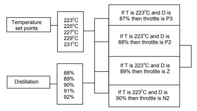
T: Temperature set point D: Percentage of Distillation FIGURE 3.3.4:Fuzzy rules for the temperature set point 223°C
