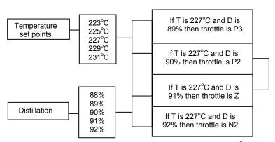
FIGURE 3.3.6: Fuzzy rules for the temperature set point 227°C
