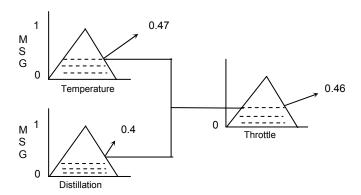
Graph 3.3.4: The two outputs are then defuzzified by center max-min rule
