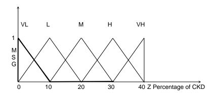
FIGURE 2.2.5: Aggregated output and defuzzificztion for the percentage of CKD
